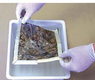
3. Bring both corners together so the film now resembles a sling. Lay the film in the center of your dipping container and easily lay both corners down together.
