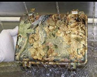
Hot or warm water is the quickest method to rinse with. After you have processed your part you will need to remove the PVA residue from the part.
